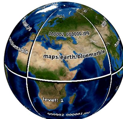
Zooming in at this view, more details need to be displayed. The tiles shown in the two screenshots above are too coarse then; Marble automatically recognizes this and changes to the next tile level where images provide more details. This keeps going: The more you zoom in, the higher the tile level. The following sketch illustrates the different number of tiles (colored) corresponding to the same map region at different tile levels:
