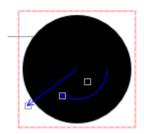
When a rigid body (here a disk) is selected you see three grey handlers on it. Using them by clicking on them and moving them, you can change the velocity, the angle and the angular velocity of the body.
