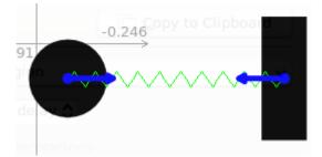
In the experiment you have a disk and a box linked by a spring. A flat box at the bottom will make a boundary. The disk and the box both have a linear motor applied to them. Two controllers allow you to change the force value of each motor. Start the simulation and play with the controllers. Then stop the simulation and add a weight force in the world (forces are global and apply to the whole world). Restart the simulation and analyze the difference.
