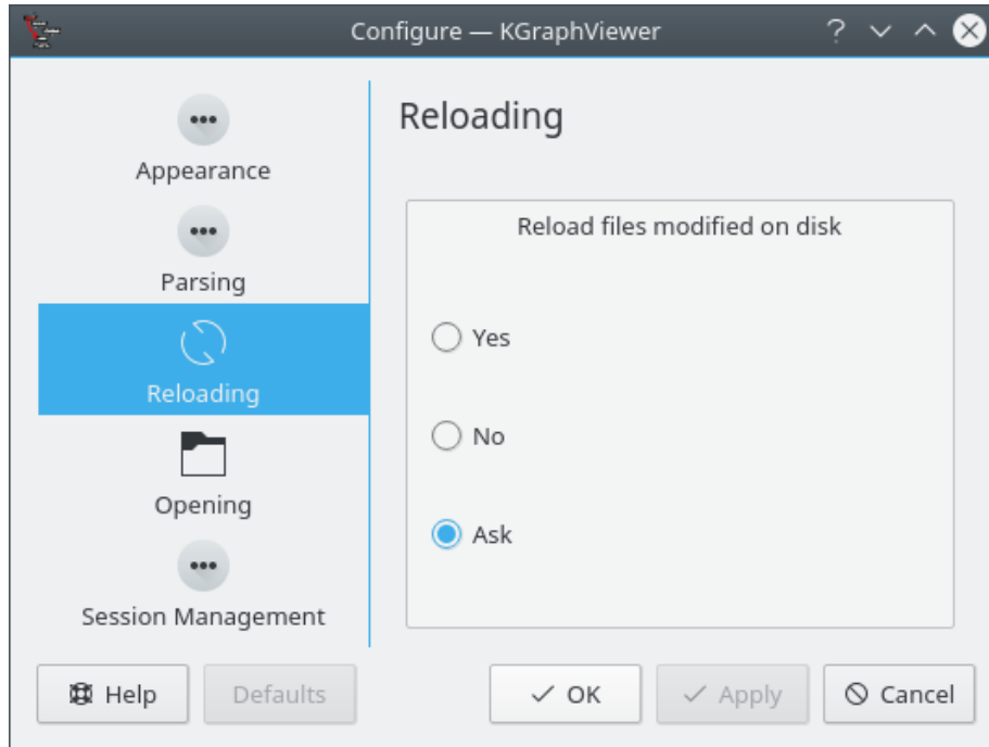
Page to reload files modified on disk in the configuration dialog
