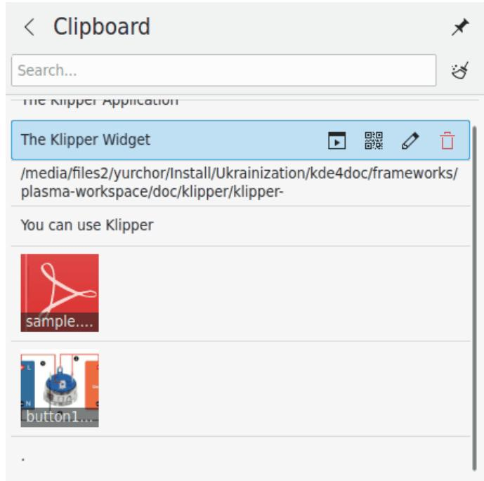
Hover an entry with the mouse pointer and four icons appear which enable you to invoke an action, show the barcode, edit the content or remove the entry from the history. Use Spectacle to capture the barcodes and save them.
