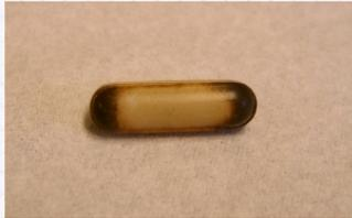
Magnetic stir bars are highly chemically inert, small magnetic bars. Most heaters have a built-in magnet which can rotate: this causes the stir bar to rotate and the mixture to become homogenized.
